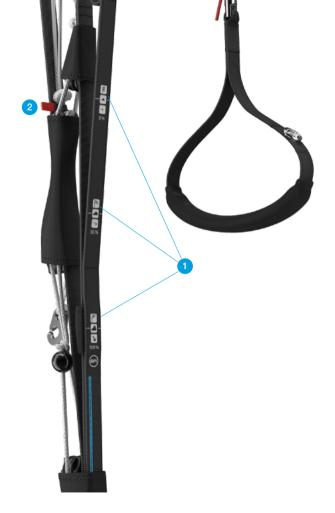
SPI at 0 %/ indicates neutral position (no accelerate).
